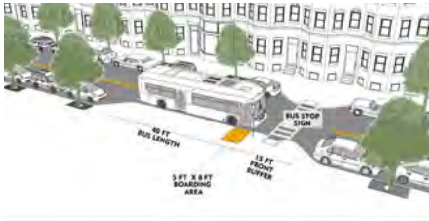
Figure 37: Mid-block boarding bus stop
