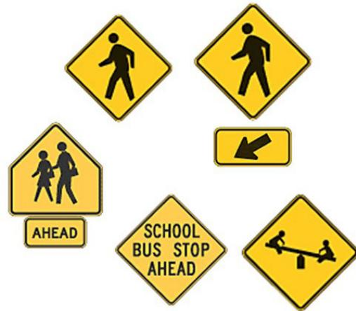
Figure 42: Example of proper pedestrian warning signage.
