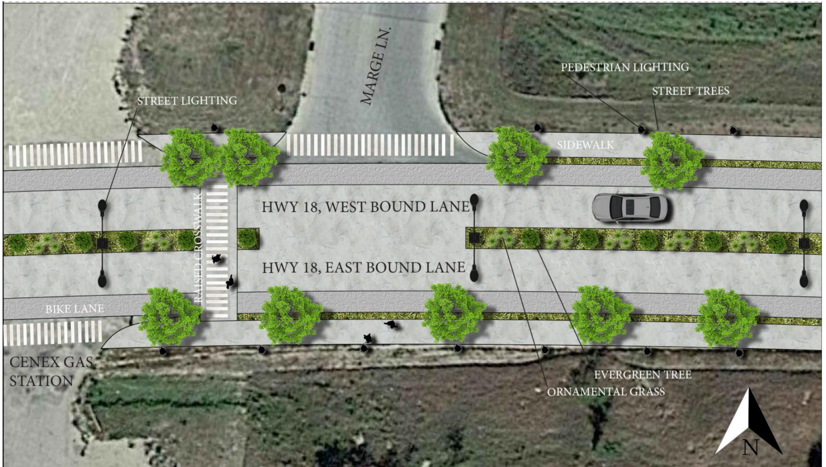
Figure 27: Plan-view of traffic-calming and pedestrian improvements, Highway 18 @ Marge Lane
