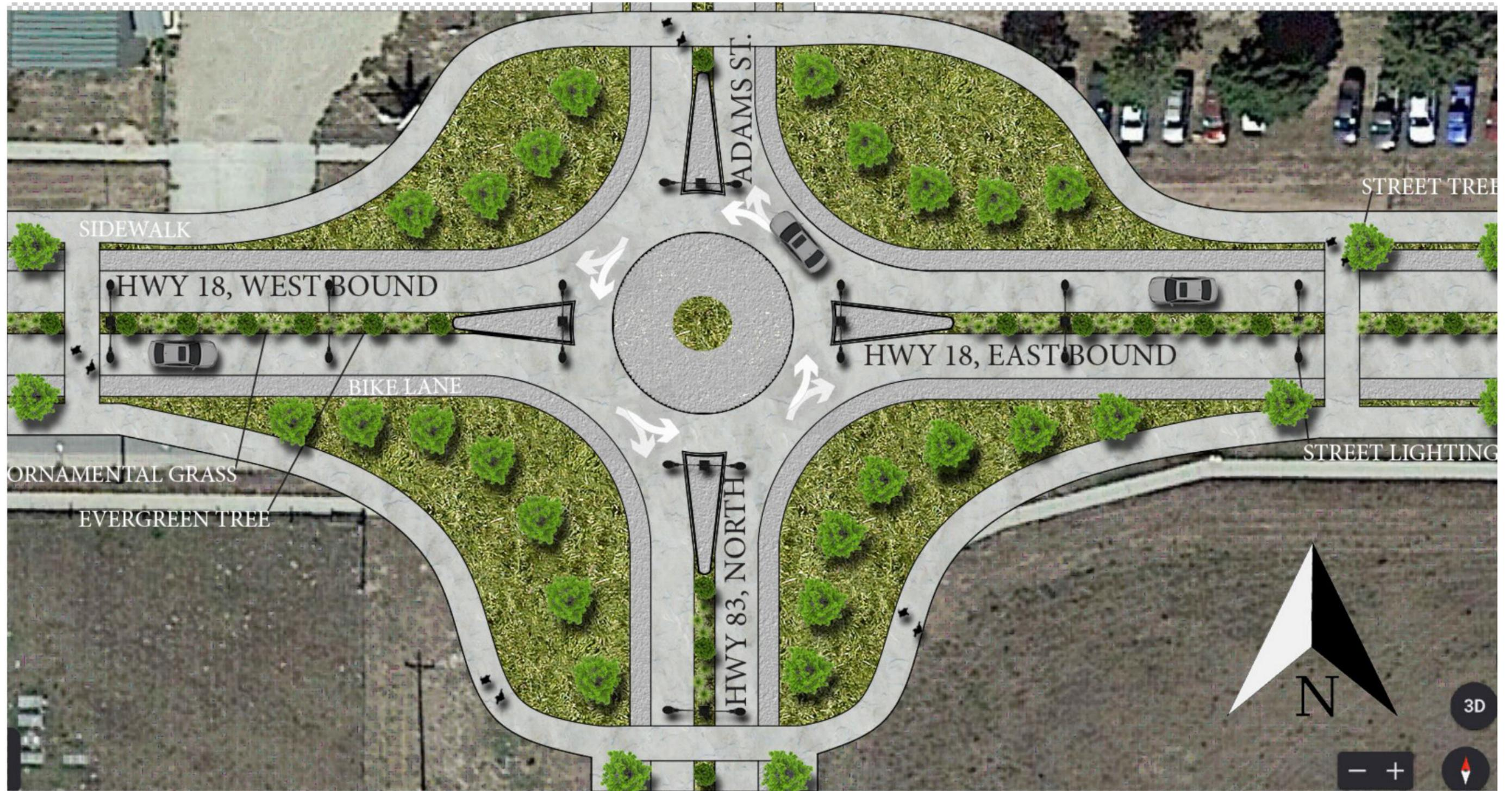
Figure 32: Roundabout design for Highway 18 @ Highway 83
