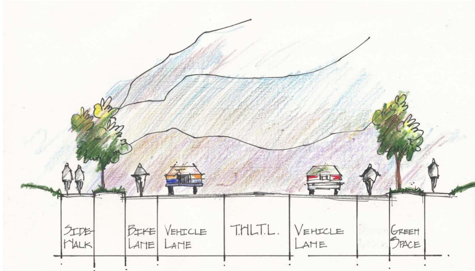
Figure 1. Road section with bike lanes and T.W.L.T.L
