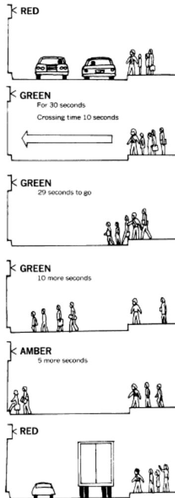
Figure 19. Intersection with Traffic Signal
